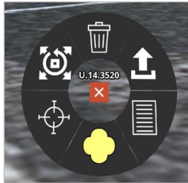
FIGURE 64. CONTEXT OPTIONS SHOWN FOR A 2525 POINT. OPTIONS ARE TO (CLOCKWISE) DELETE, SEND, SHOW DETAILS, CHANGE TYPE, PLACE SPI , AND TRANSLATE (MOVE)
