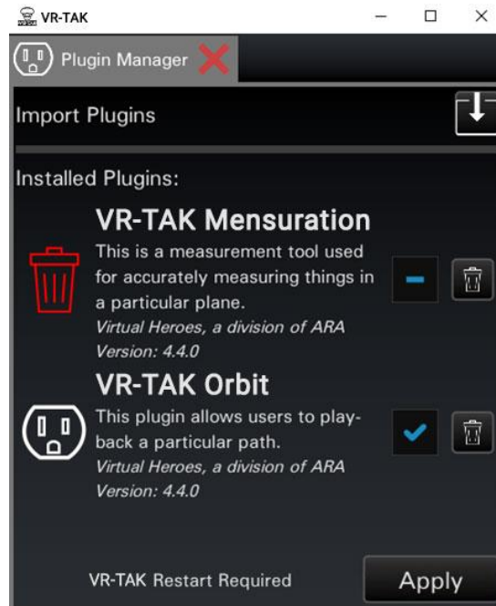
FIGURE 55. PLUGIN MANAGER UI. VR-TAK MENSURATION HAS BEEN MARKED FOR DELETION AND WILL BE REMOVED WHEN THE APPLY BUTTON IS CLICKED. ADDITIONALLY, VR-TAK ORBIT HAS BEEN ENABLED AND WILL BE LOADED INTO VR-TAK WHEN THE APPLY BUTTON IS CLICKED
