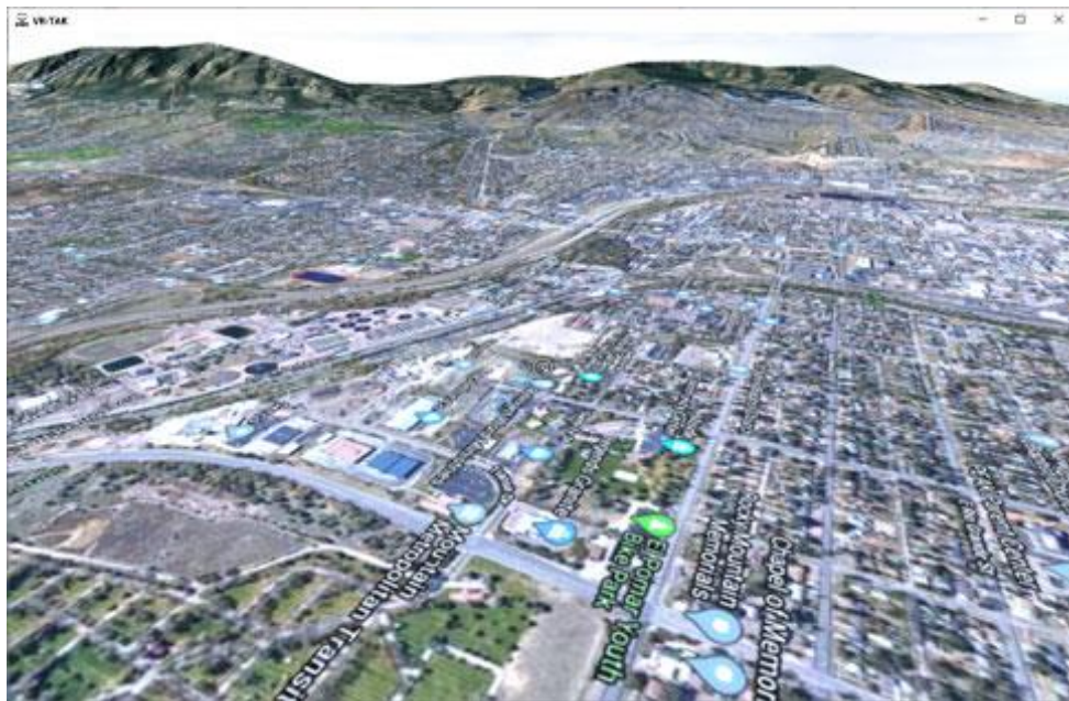
FIGURE 125. TERRAIN TILE OF COLORADO USING GOOGLE HYBRID AND DTEDO
