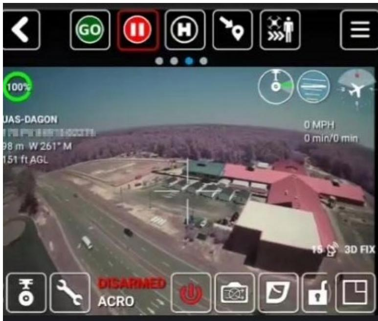
*Note the absence of VTX OSD from DJI Goggle V2 video out. Also, mix of telemetry from the Betaflight aircraft (eg: disarmed but in the air)*
